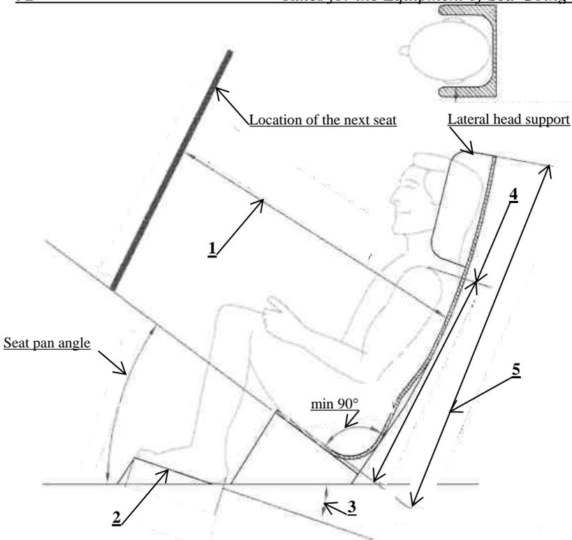
Fig. 6.16.2.2 Parameters and layout of the seat in a free-fall lifeboat.
