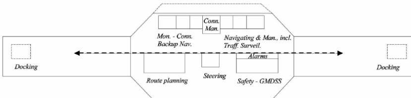
Рис. 2.5.17-3 Design principles — Flat front — Open bridge wings with passageway from door to door Consoles up front — Access to front window.
