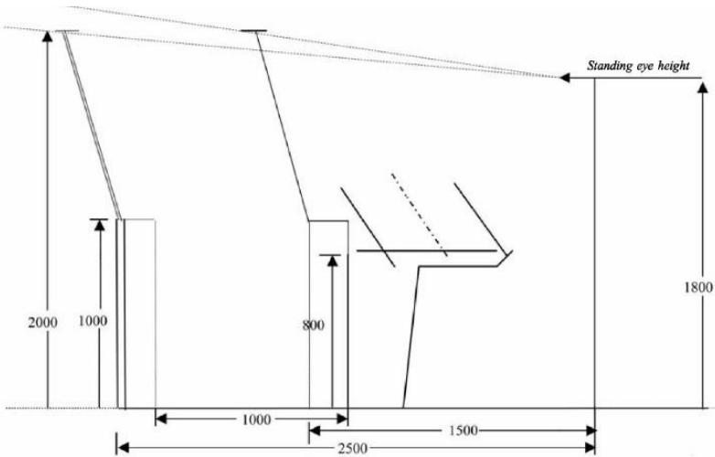
Fig. 2.6.3 With front windows at an angle of  $15^\circ$ , a vertical angle of view of  $5^\circ$  from an eye height of 1750 mm may be provided at a distance of 2600 mm from the front bulkhead, all owing for a passageway of 1000 mm in front of workstation consoles.
