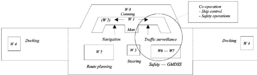
Fig.5.1.2. Design principles — Location of workstations Enabling efficient bridge team management during different operating conditions.
